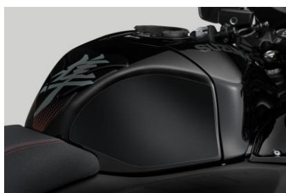
19 Fuel tank protection sticker
