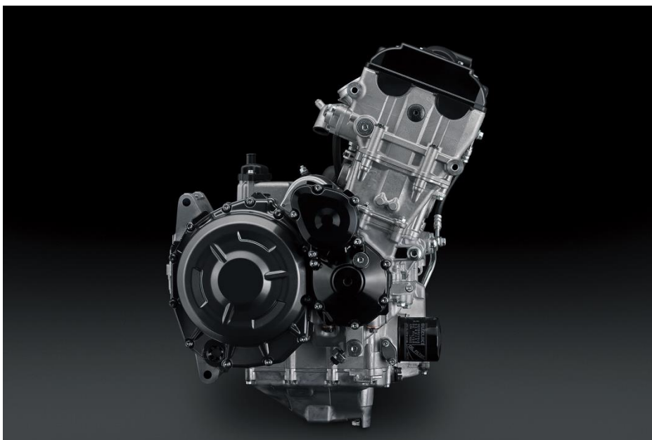
4-stroke, 4-cylinder, liquid-cooled, DOHC, 1,340cm 3 engine
